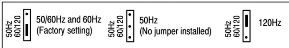
The control can also operate 60 Hz and 50/60 Hz motors (not 50 Hz motors) in an over speed mode. Note: In this mode, motor will produce full rated torque up to 60 Hz. Above 60 Hz, torque will linearly reduce to 50% at 120 Hz.
