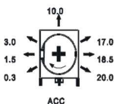
**Application Note:** On applications with high inertial loads, the deceleration may automatically increase in time. This will slow down the rate of speed decrease to prevent the D.C. bus voltage from rising to the overvoltage trip point. This function is called regeneration protection. It is recommended that for very high inertial loads that both the ACC and DEC trimpots be set to a minimum of 10 seconds.
