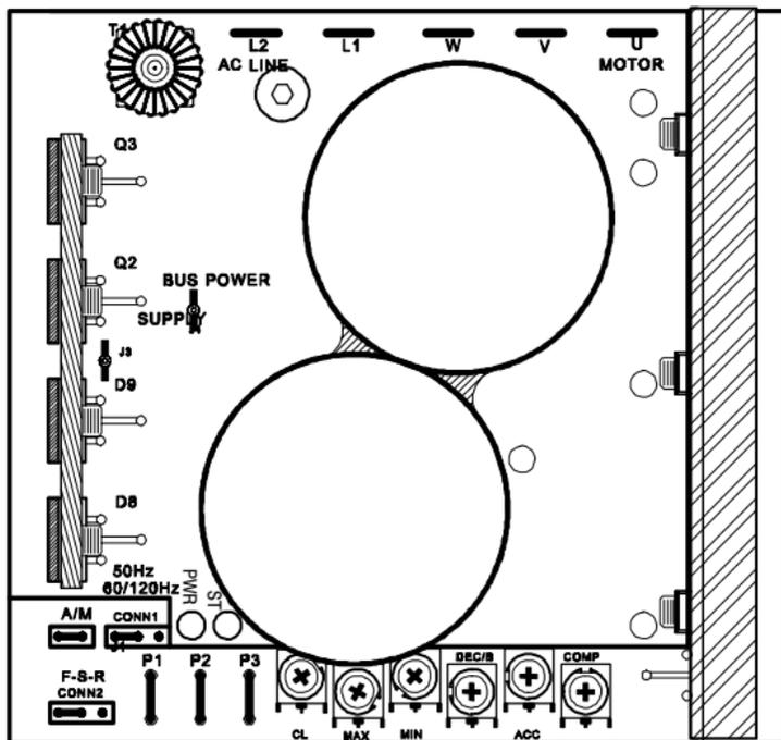
FIG. 3A – SERIES 5 Inverters 1/2 HP Mechanical Specifications – Inches / [mm]
