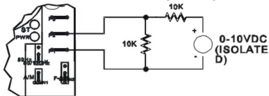
Note: For proper operation, “MIN” trimpot must be turned to zero (CCW). If 0-10VDC operation is required, a resistor network can be added as per fig. 6C. If an isolated signal is not available, a separate signal isolator must be used (BC145 or equivalent). Do not ground (earth) signal wiring.
