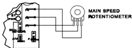
Fig. 6B – Signal Following 0-5VDC (Isolated)
