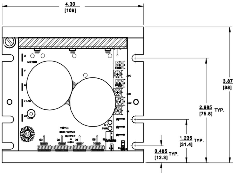
FIG. 3B – SERIES 5 Inverters 1/2 HP Mechanical Specifications – Inches / [mm]
