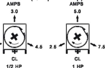
1. Connect an AC ammeter in series with one motor phase.
